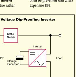
than a curative solution. It consists of a static switch in series with, and an inverter parallel to, the load. Switch over occurs in 600 µs. Since energy is stored in a capacitor instead of a battery, there are no replacement costs, maintenance costs, or hazardous waste.
